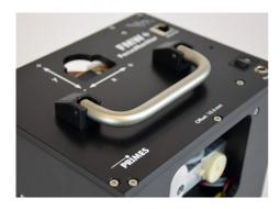
The FMW+ is an opto-mechanically scanning measuring system that scans the laser beam with a special measuring tip. This is provided with a small hole (typical diameter 20 µm) that lets through a small section of the laser beam.
